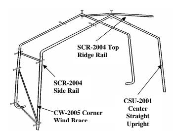
**Step 5**. Begin the Top Ridge Rail by placing a Swedged Cross Rail <u>underneath</u> the End Top Crest Tube. Secure the Cross Rail loosely with a Carriage Bolt#CBN-3000-2 with washer and nut facing the interior of the unit.
