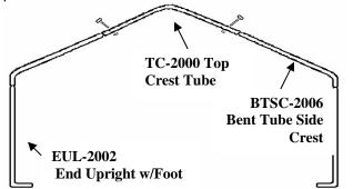
**Step 2**. Assemble the (2) Corner Wind Braces #CW-2005 to the End Upright w/Foot #EUL-2002 to the first of the End Arch assemblies. Use a #CBN-3005-3 Carriage Bolt with Washer and Nut to secure the braces loosely to the Upright. Do not tighten completely.
