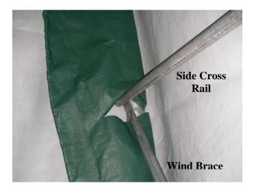
When putting on the doors, adjust the length to make certain the doors do not drape onto the ground. Adjust door length by pulling more or less fabric over end arch. If pulling them up puts too much stress on the slit where it goes over the wind brace, use a sharp knife to cut slit another inch or two to relieve it. The PE fabric is rip-stop weave, and can easily be cut to relieve stress at the frame members.
