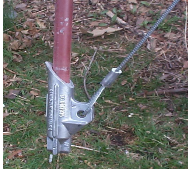
Drive Rod inserts into Anchor Head
